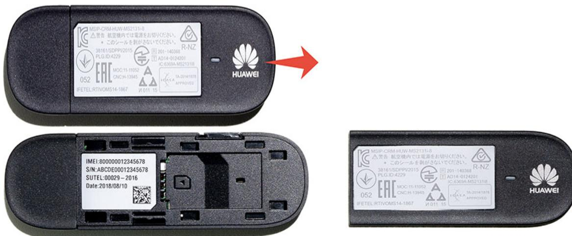
3. **Insert the SIM card** into the slot as shown below, making sure that the angled corner of the SIM card is oriented correctly. When fully inserted, the SIM card logo should remain visible.
